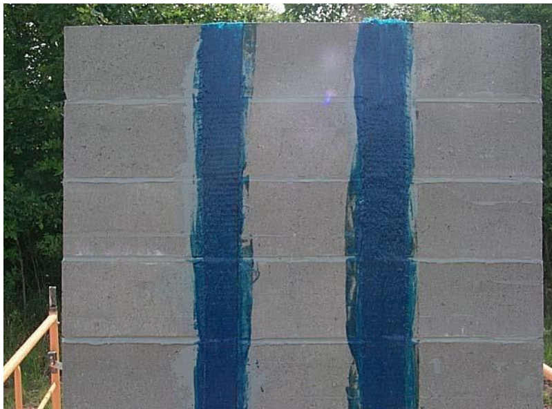
Hybrid System including FRP Rods and Sheets
