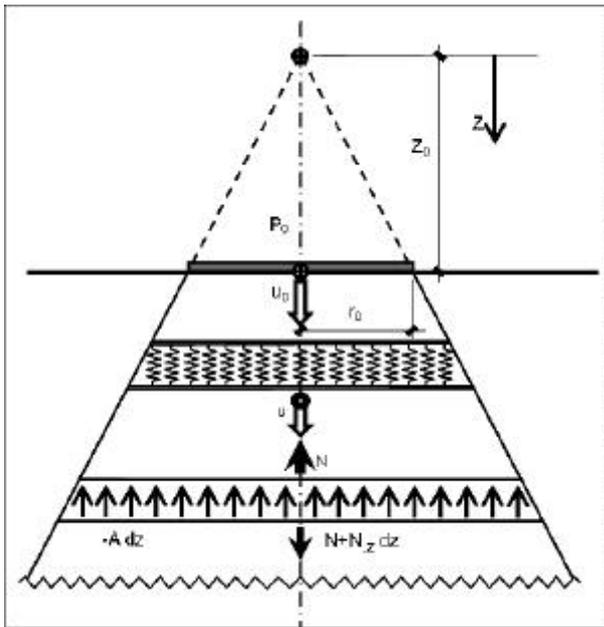
Figure 2. Soil model based on cone model.
