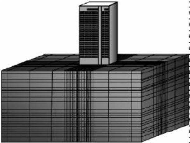
Figure 1. Finite element model of soil structure system.
