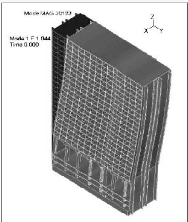
**Figure 4.** Three dimensional finite element of the Azadi hotel structure.
